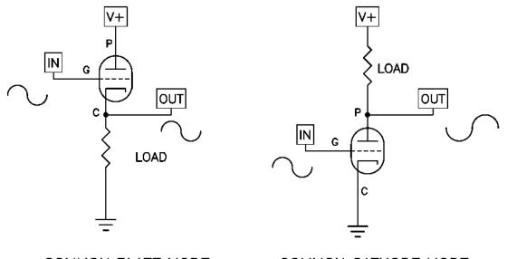
COMMON PLATE MODE (CURRENT GAIN ONLY) COMMON CATHODE MODE (VOLTAGE + CURRENT GAIN)
