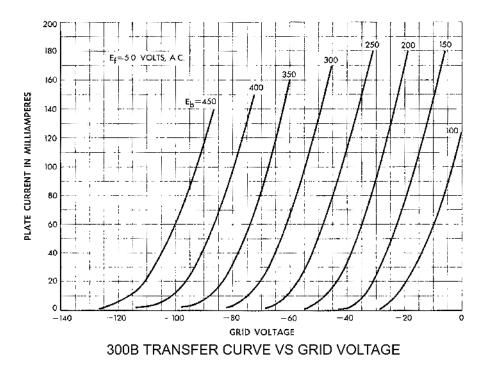
Looking at this curve, we see that the lines are curved – the more current, the faster they rise. Below is a different view of the same character, but with the current plotted as a function of the Plate voltage with each line representing a fixed value for Grid voltage.
