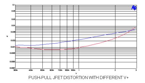
Here's a technique we use at Pass Labs – the use of some single-ended bias in a push-pull output stage to reduce distortion. The distortion curve below shows what you can get if you simply put a small value current source in parallel with one of the JFETs as shown on the middle circuit. The current source displaces the bias current values on the JFETs until they achieve a more perfect distortion cancellation:
