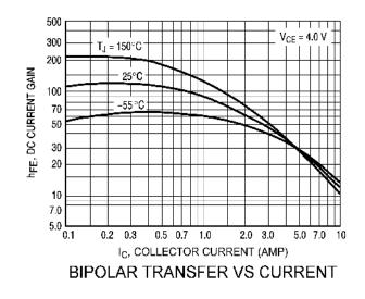
There is also a dependence on Vce known as the Early effect, a slightly straight line dependency increasing with voltage. As with other devices, finding the sweet spot for a bipolar device means locating the point where these variations result in distortion cancellation.
