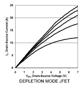
You will note that these aren't the tiny little signal JFETs that everyone is accustomed to. These are examples of the new generation of high power JFETs coming out of the labs. In the 1970's when Yamaha and Sony produced power JFET devices for use in their own amplifiers it created some excitement among audiophiles. Unfortunately it seems that they were ahead of their time, and now those parts are quite rare.
