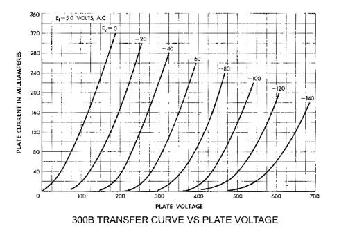
These lines are also curved with a shape very similar to the previous graph. A perfectly linear tube will have these lines in both graphs perfectly straight and equally spaced. Any deviation from that would be distortion. Looking at the curved lines, we can see that there is quite a bit of distortion.
