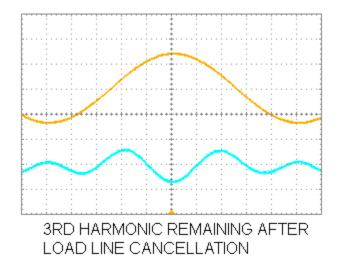
If your criteria instead is a particular harmonic content and/or harmonic phase, a deviation from this point in either direction will give you second harmonic back with its phase depending on which way you went, and you can tweak this in relation to the amplitude of the third harmonic if you like.
