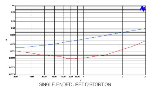
Alternatively we could have adjusted the bias current or the load resistance, and we also could have tried for best performance at some higher voltage that 1 volt.
