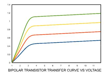
Here we see the gain vs current curve of an NPN power transistor showing some gain dependence vs Collector current. Above a couple of volts, the variation is much less and forms a fairly linear straight line with voltage.
