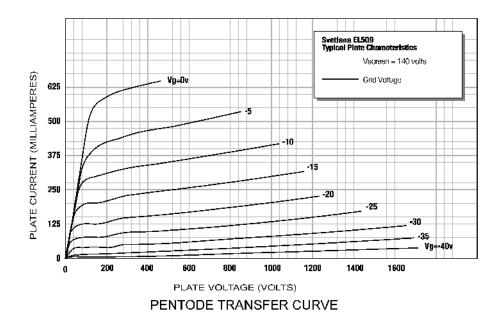
Here we see a family of curves which indicate that the gain (transconductance) increases exponentially with Plate current, but has less variation with respect to Plate voltage as compared to the Triode. You can still vary the voltage, current and load parameters to find the sweet spot, but it will be in a different place.
