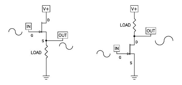
COMMON DRAIN MODE (CURRENT GAIN ONLY) COMMON SOURCE MODE (VOLTAGE + CURRENT GAIN)
