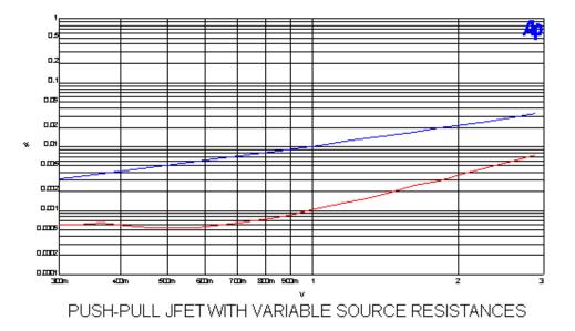
Here we see that a simple adjustment of the pot can drop the distortion by 90% without having significant effect on the other aspects of performance.
