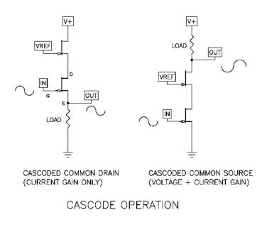
It's pretty easy to get into the sweet spot using a cascode, and if you want to explore this in some more detail, I recommend Zen Variations 9, which you can download from <u>www.passlabs.com</u>. There we explore getting the lowest possible distortion from an amplifier using a single stage with a power JFET having a high current rating, but a low voltage and dissipation rating.
