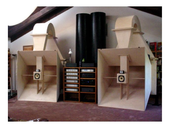
El Pipe-O is basically two big lengths of 24 inch diameter Sonotube with 21 inch woofers at the bottoms and damped with Dacron or Polyfill. They easily go down to 20 Hz, but their transient characteristic is not so good up around 100 Hz, so you can imagine them as an ideal match. Any room that can hold KleinHorns can find some space for El Pipe-O, and the over-the-top approach tends to appeal to the same builder.
